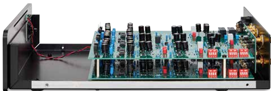
ABOVE & LEFT: Dual mono crossover boards are configured for two- or three-way operation. DIP switches [red] set the input level matching, not crossover points. Umbilicals carry DC power to two sockets
